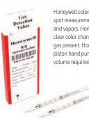
Honeywell colorimetric gas detection tubes enable guick, on-thespot measurement of a wide range of toxic and combustible cases and vapors. Honeywell tubes are easy to read, and provide a sharp, clear color change directly corresponding to the concentration of gas present. Honeywell tubes are compatible with the Honeywell piston hand pump, a reliable way to draw samples of an exact volume required for the most accurate measurements.
